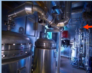
LMBV Schwarze Pumpe Germany, 5 MPPE units, 75 m3/h; Ar, Al, PAHs
